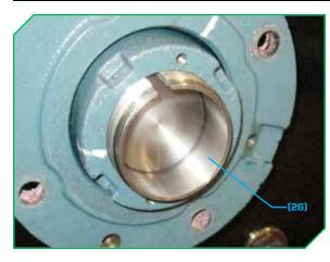
**25** Push the adapter sleeve<sub>(26)</sub> insert in as far as possible (towards the drive side bearing).
