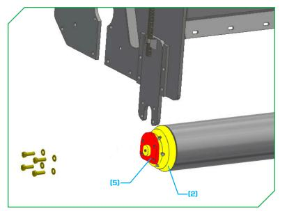
Slide the retaining plate<sub>(5)</sub> onto the bearing shaft<sub>(2)</sub> in the orientation illustrated for the non-drive belt side of the flail.
