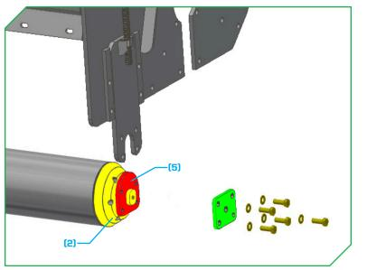
Slide the retaining plate<sub>(5)</sub> onto the bearing shaft<sub>(2)</sub> in the orientation illustrated for the drive belt side of the flail.
