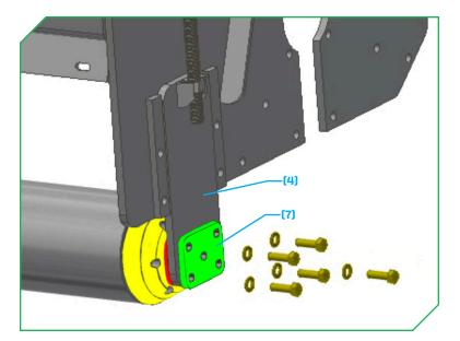
Place the mounting plate<sub>(7)</sub> over the mounting holes of the cutting height adjustment plate<sub>(4)</sub> on the drive belt side of the flail
