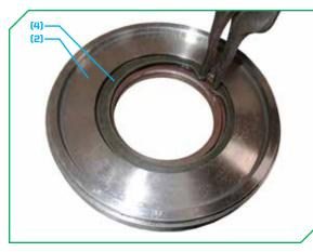
Remove the small spring retainer ring<sub>[4]</sub> on the back side of the seal holder<sub>[2]</sub>.
