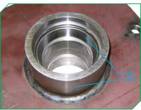
Position the spindle housing<sub>(14)</sub> upside down so the bottom of the spindle housing<sub>(14)</sub> is exposed, and insert the lower bearing cup<sub>(3)</sub>.
