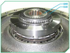
Slide the splined insert<sub>(22)</sub> into the splines on the inside of the output shaft<sub>(13)</sub> as illustrated.
