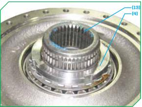
Thread the lock nut<sub>(4)</sub> onto the output shaft<sub>(13)</sub> threads (conical / tapered side down) until it contacts the lock washer<sub>(15)</sub> underneath.
