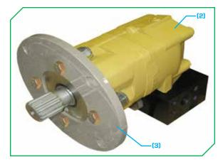
• Low flow motors<sub>(2)</sub> utilizing a spacer<sub>(4)</sub> will have the spacer<sub>(4)</sub> mount between the low flow motor<sub>(2)</sub> and the spindle, utilizing the motor mount hardware.
