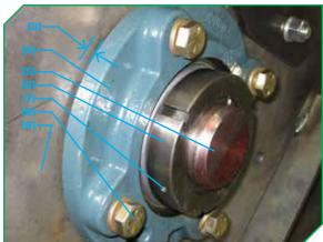
**NOTE:** A spanner wrench<sub>(1)</sub> (part #24-0110 - used for bearing #10-0002) and spanner socket<sub>(2)</sub> (part #24-0109 - used for bearing #10-0006, part #24-0111 - used for bearing #10-0057, part #24-0113 - used for bearing #10-0059) are recommended for tightening grip-tight bearings. Contact Diamond Mowers Inc. to order these tools.
