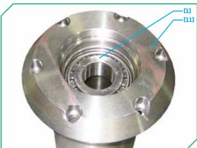
• Turn over the ground roller insert<sub>(11)</sub> and place a taper bearing<sub>(1)</sub> into the taper bearing race<sub>(2)</sub> on the face side of the ground roller insert<sub>(11)</sub>.
