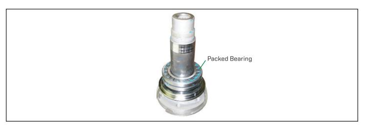
7. Place the spindle housing down around the spindle shaft until fully seated.
