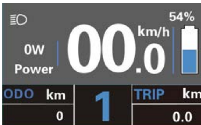
Switching the Lighting On/Off Interface
