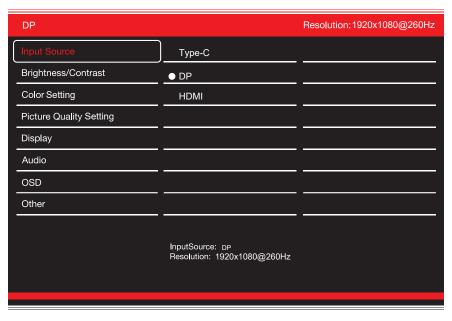
Switch the signal input to Type-C, DP, HDMI, or have the monitor Auto Select the source.
