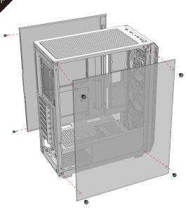
Glass side panel installation: fix the glass side panel with 4 screws (as shown above)
