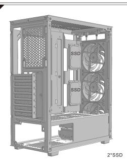
Align the screw holes of the hard disk with the hard disk bracket and fix it with special screws.
