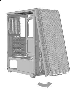
To remove the front panel of the case, pull it by hand, firmly from the bottom of the panel
