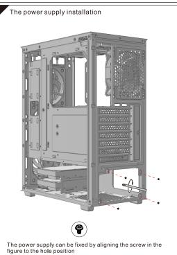
Note: different types of power supply, hole location may be slightly different, take the actual object as the standard
