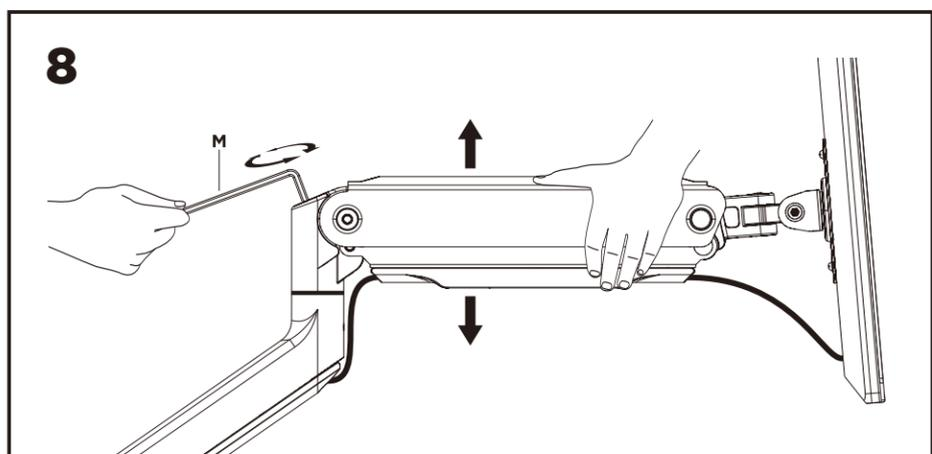
To properly balance the arm with monitor mounted, adjust the spring tension using the supplied Allen Key as follows:
