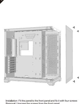
Installation: Fit the panel to the front panel and fix it with four screws Removal: Unscrew the screws from the front panel
