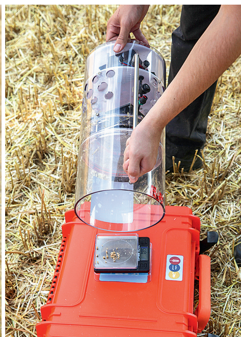
Steps to measurement, left to right: Pour chaff and grain from the trays into the battery-driven separator; use it to winnow chaff; and then weigh the remaining grain. Fan speed is adjustable to suit the crop. The unit's handle and screen have now been changed to make them more user-friendly.
