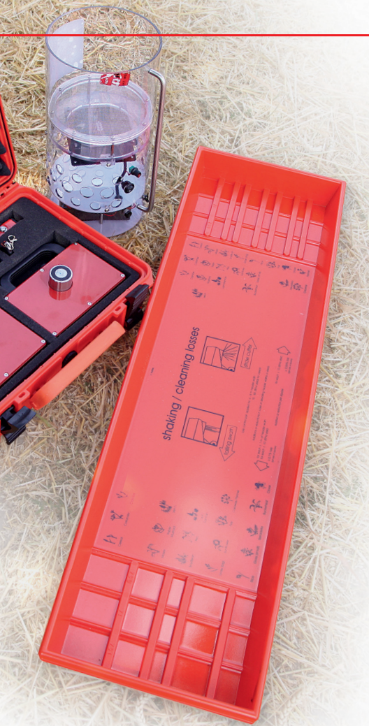
The LMS kit has two remotely operated tray release units (in case, left), a battery-powered separator (top) and three collecting trays.
