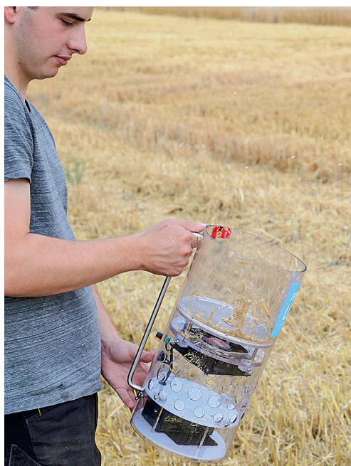
Steps to measurement, left to right: Pour chaff and grain from the trays into the battery-driven separator; use it to winnow chaff; and then weigh the remaining grain. Fan speed is adjustable to suit the crop. The unit's handle and screen have now been changed to make them more user-friendly.
