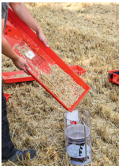
Steps to measurement, left to right: Pour chaff and grain from the trays into the battery-driven separator; use it to winnow chaff; and then weigh the remaining grain. Fan speed is adjustable to suit the crop. The unit's handle and screen have now been changed to make them more user-friendly.
