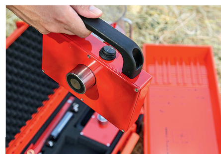
The release solenoids run off battery power, so you need to remember to switch them off after use.
