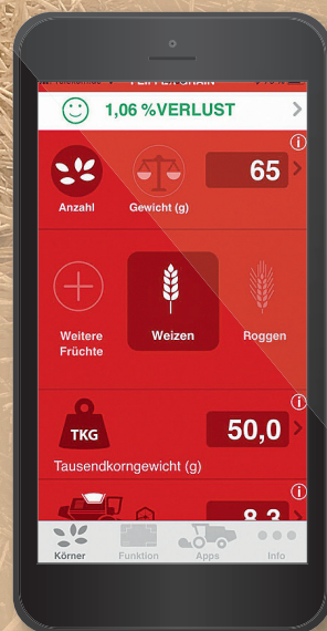
Feiffer's Grain Tablet (left) and its companion app take much of the guesswork out of combine loss measurement.
