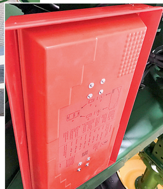
On this John Deere T660i harvester, the tray release plate found a home just in front of the back axle. A pair of electromagnets then holds the tray until it's released on the move by the combine's operator.
