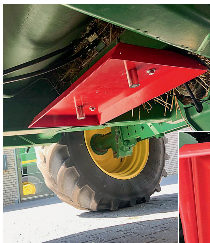
On this John Deere T660i harvester, the tray release plate found a home just in front of the back axle. A pair of electromagnets then holds the tray until it's released on the move by the combine's operator.
