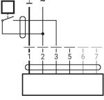
Connection with switching contact Connection with active sensor
