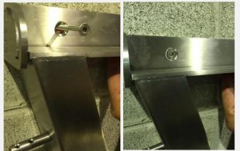
8. Fold both frames up and loosen all 24 grub screws with Allen key provided ready for cable placement.
