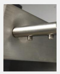
9. Slide end of cable in first fitting starting from the front fitting and ensure the cable is all the way in and tighten down both grub screws.
