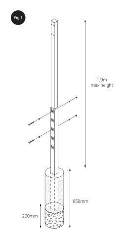
1.4 Adjust the Post Kit until the desired height is achieved. The top of the Top Post should be 115mm above user head height. (refer to your Retracting Clothesline manual).
