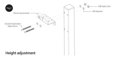
3.1 Your Post Kit has three height positions for a total of 236mm adjustment. To adjust the height of the Top Post, remove bolts, washers and nuts and move to new position. Re-secure bolts, washers and nuts. (Figure 3)
