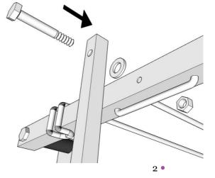
Repeat this bolt configuration, this time attaching the stay to the low line arm directly under the main arm. Secure with a nut. Repeat on the opposite side.
