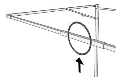
**Warning:** Do not continue to lift the bar past the engaging point (struts clicking) as this will break the strut mechanism and a new strut will be needed at the cost of the consumer.
