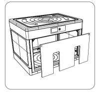
Open the front door and stick the front of the cup tunner into the curing machine.
