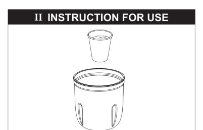
1.Take off the head, put the mixed resin cup into the container. Do not mix resin too full. Otherwise, it may spill out while vacuuming or bubbles may be stuck inside due to resin overheating.
