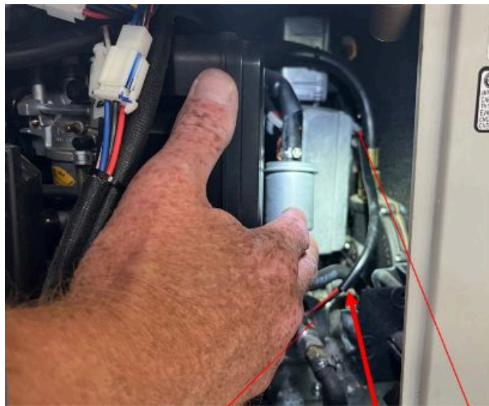
Fuel pump Fuel pump wire harness Cut fuel pump wires here and butt splice in the wires for the new fuel pump
