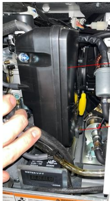
Airbox cover securing screw
