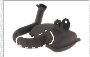
SIP Road for Vespa PX200 with diffuser (extends into the body!)
