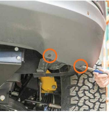
4. Use a T-30 torx to remove the 2 bumper bolts located next to the radiator support.
