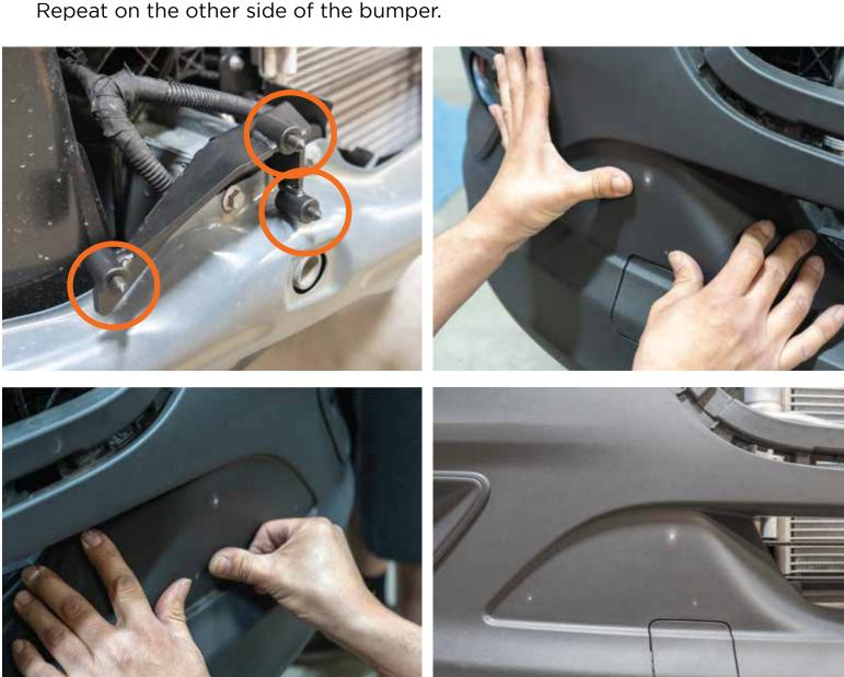
12. Remove the 2 T-30 torx upper bumper bolts and detach the bumper cover.
