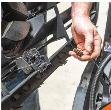
3. Use a panel clip removing tool to remove the 6 push pins attaching the driver's side forward-facing front inner fender liner. Repeat this step on the passenger's side of the vehicle.
