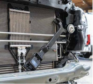
7. Use a 13mm socket to remove 3 out of 4 bolts holding the crash bumper on each side. Then loosen, but do not remove, the remaining 2 bolts holding the crash bumper.
