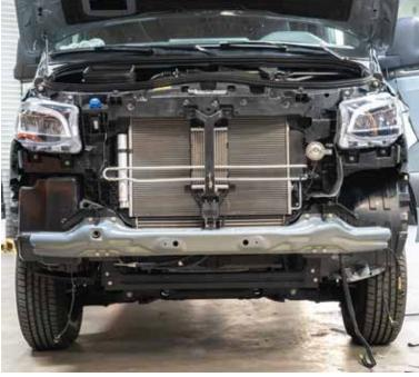
14. Reconnect the parking sensor & fog lights harnesses to the vehicle before installing the bumper cover. Use the 2 T-30 torx upper bumper bolts to keep the bumper in place. Do not fully tighten them yet. Push the bumper cover clips back into place, starting under the headlights and working out to the sides of the vehicle. Then fully tighten the 2 T-30 torx upper bumper bolts.
