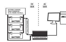
**Note:** For safety purposes, you can connect a DC-rated fuse or DC-rated circuit breakers on the positive cable line in your power system, following recommendations below.
