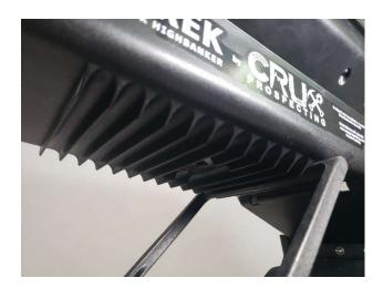
At this time, ensure that your damper is set correctly and not stuck in the sluice mat or folded under the hopper diverter.
