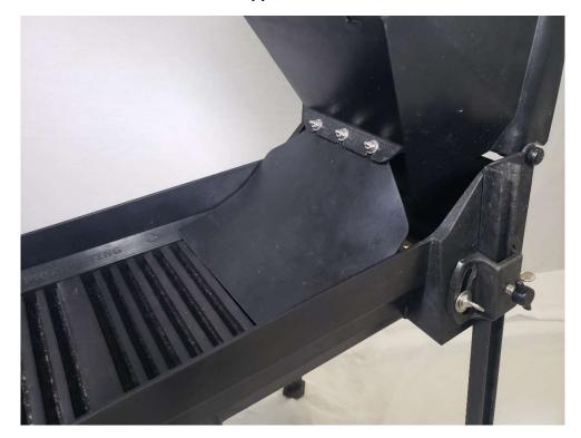
Looking at the inside of the hopper, you can see the textured pattern that helps direct material to the center. You can also see the 2 holes for the grizzly screen tabs as well as the top side of the large material diverter.
