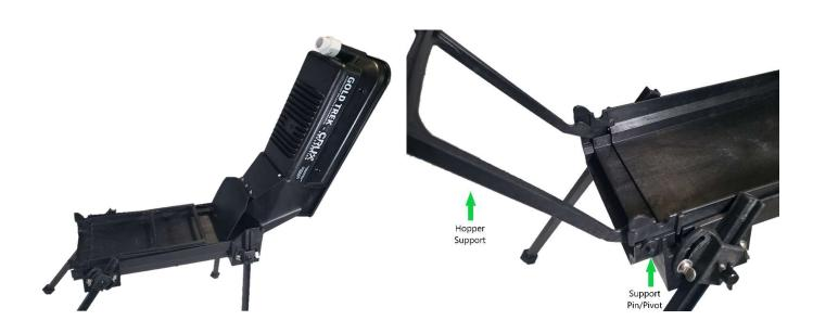
Once you've identified the support pins, flex one side of the support arm inward to remove the pin from the base. When one side is out, tension on the arm can be released. Remove the other side's pin to fully separate the support from the system and set aside.
