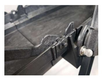
With the hopper support now locking the sluice pieces together and the hopper still pivoted out of the way, we can now install the sluice mat. Start by sliding the first mat under the pre-installed mat strip. Make sure it's lapping correctly and pressed tightly into position.
