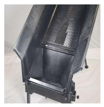
Choose a grizzly screen, either 3/8" or 1/2" classification. Line up the tabs of the screen to the receiving holes in the floor of the hopper. Insert the screen into the receiving section at an angle and press down to lock into place.
