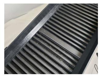
With your sluice matting fully installed, pivot the hopper to engage the notches on the bottom of the hopper with the hopper support arm. Select the notch to adjust the hopper pitch depending on personal preference or paydirt composition.
