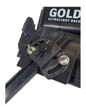
Once the legs are installed, stand the system up. You can now identify the hopper support arm which is installed between the nested sluice sections. The pivot pins through the walls of the base are designed to be under tension to lock the two sluice sections together when packed.
