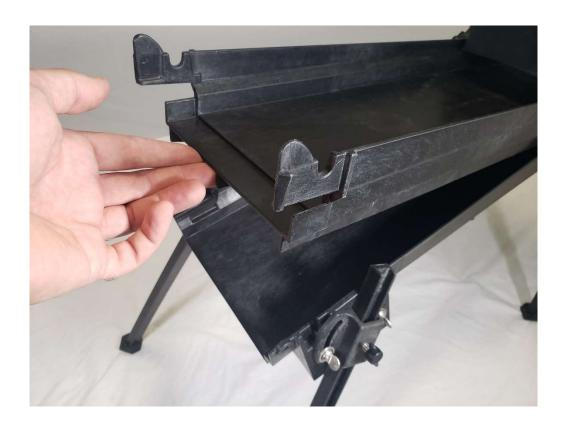
With the lower sluice section removed, turn it 180 degrees and line up the tabs to connect it to the base. The tabs are designed so they must be flexed inward slightly to fit inside the base walls. The lower under lap area will go under the base of the sluice floor.
