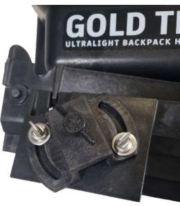
Insert all 4 Legs into the 4 corner brackets and tighten the center black toggle. You may need to pull up on the black toggle to seat the nut on the inside. Take care not to loosen the toggle too far or the inside nut may fall out. Some people choose to epoxy or glue this nut inside the bracket if they are concerned about losing parts.
