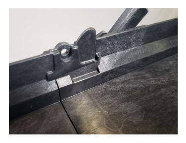
Once the sluice sections are locked together, you may reinstall the hopper support by inserting one side's pin through the base wall and flexing the support arm to allow insertion of the other side.
