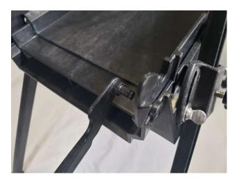
With the support arm removed, you may now lift the nested lower sluice section and remove it from the base.
