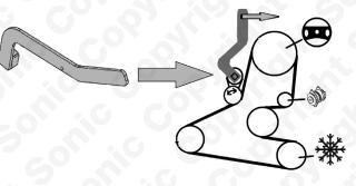
Component 5 - Camshaft Alignment Strap
