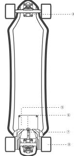
Max. Speed: 45km/h Max. Climbing Grade: 30% / 16.8° Range: 25km Gross Weight: 7.3±0.2kg Torque: 5.2Nm × 2 Maximum Power: 1500W × 2 Rated Motor Power: 750W × 2 Rated Charger Power: 75W Input Voltage: 100-240VAC,50/60Hz Battery Capacity: 193Wh Charging Time: 2h 45min Truck: Seismic Aeon 45° Braking Mode: Regenerative Braking Applicable Age Range: 16 ~ 50 Years old Maximum Load: 200kg / 440lbs Water Proof Level: IP55
