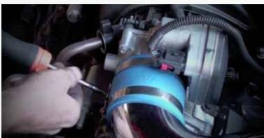
Loosen the clamps on the air intake tube and air box, and then remove the tube.
