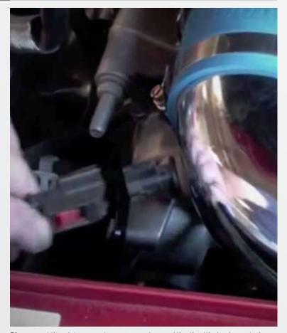
Disconnect the air temperature sensor plug and the throttle body control motor plug.
