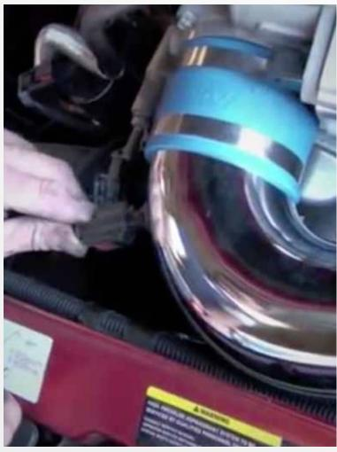
Re-connect the air temperature sensor and the throttle body control motor plug. Re-connect the negative battery terminal and refer to page 2 of the instruction sheet for throttle relearn procedure.
