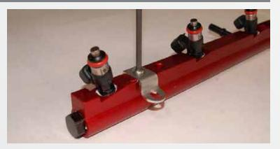
Install the supplied mounting brackets onto the bottom of the BBK Fuel Rails using supplied 1/4"-20 button head screws. Use the holes marked LS2.
