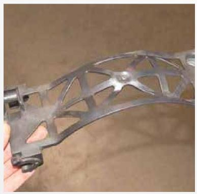
Remove the rear engine cover plastic mounting bracket. This will NOT be re-installed.
