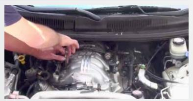
Use a 10mm socket to remove the bolts that attach the fuel rails to the intake manifold, and an 8mm socket to remove the small L shaped bracket that attaches to the fuel rail stud on the passenger side. Corvette models may require that you remove the intake manifold bolts and slide it forward to remove this bracket.
