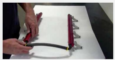
Assemble the crossover hose by pushing the barbed ends of the supplied 90° - 6 fittings into the ends of the hose.
