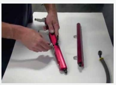
Insert (4) injectors into each rail.
