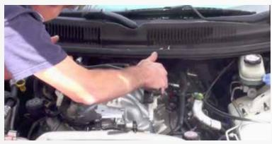
Remove the fuel rails and injectors by simply lifting them straight up.
