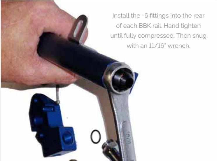
Install the -6 fittings into the rear of each BBK rail. Hand tighten until fully compressed. Then snug with an 11/16" wrench.
