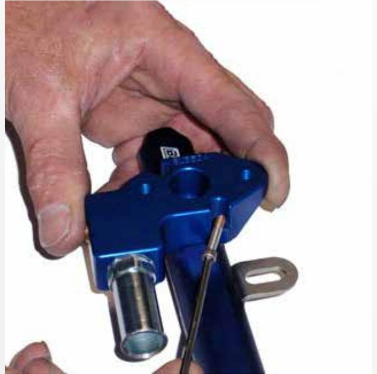
Wrap a small amount of Teflon tape around the threads of the supplied brass Allen headed block off plug, or a fuel pressure gage of your choice and thread it into the 1/8" pipe threaded port in the BBK pressure sensor mount.
