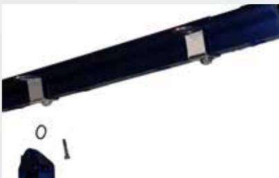
Install the mounting tabs onto the bottom of the BBK rails by placing a washer over the threads of each of the supplied 1/4"-20x 3/8" (shorter button head) Allen bolts and placing the bolt through the round hole (not the slot) in each bracket.
