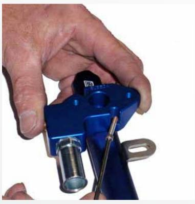
Wrap a small amount of Teflon tape around the threads of the supplied brass Allen headed block off plug, or a fuel pressure gage of your choice and thread it into the 1/8" pipe threaded port in the BBK pressure sensor mount.
