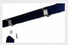
Install the mounting tabs onto the bottom of the BBK rails by placing a washer over the threads of each of the supplied ½"-20x 3/8" (shorter button head) Allen bolts and placing the bolt through the round hole (not the slot) in each bracket.
