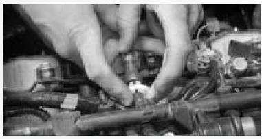
Using the 3/8" spring lock tool, disconnect the fuel rail feed hose.
