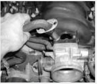
Using a 10mm socket, remove the throttle body bracket and EGR tube from the front of the intake manifold.
