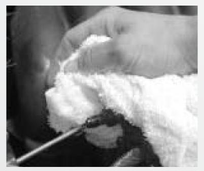
Carefully release any fuel system pressure by removing the cap at the front end of the driver side fuel rail and depressing the Schrader valve using a small screwdriver while shrouding the valve with a rag or cloth.
