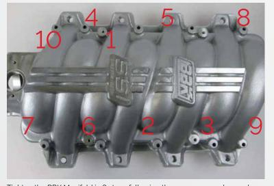
Tighten the BBK Manifold in 3 steps following the sequence as shown above until the split washers are flattened. (Do not over tighten! These bolts only need to be tight enough to compress the o-rings).
