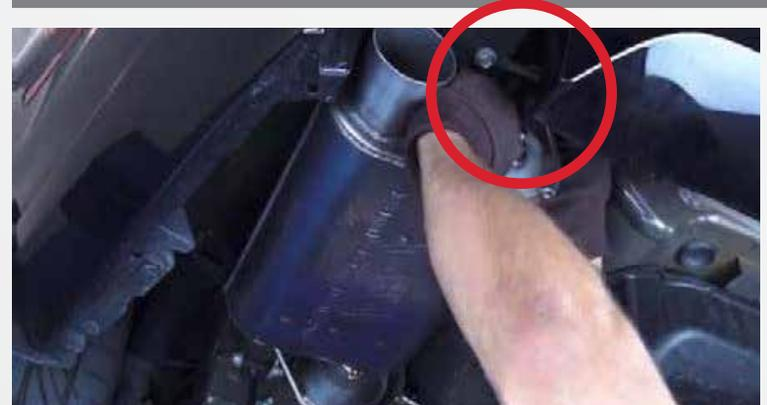
Slide the muffler over the inlet pipe, then slide the grommet closest to the rear bumper onto the muffler hanger.
