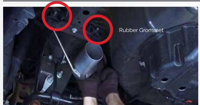
Starting on the driver side, slide the inlet pipe through the 2 hanger grommets and into the mid pipe and snug the clamp to hold the tubing in place.
