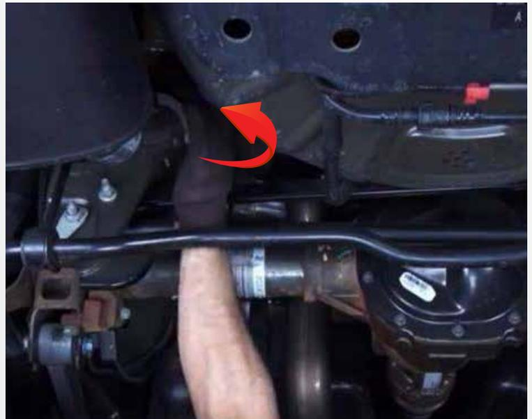
Twist the mid pipe so the muffler has enough clearance to be removed.
