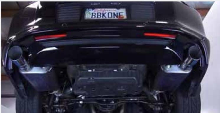
With all the clamps snug, make any fitment adjustments starting at the front clamps on the mid pipe and ending at the muffler tips, then tighten.
