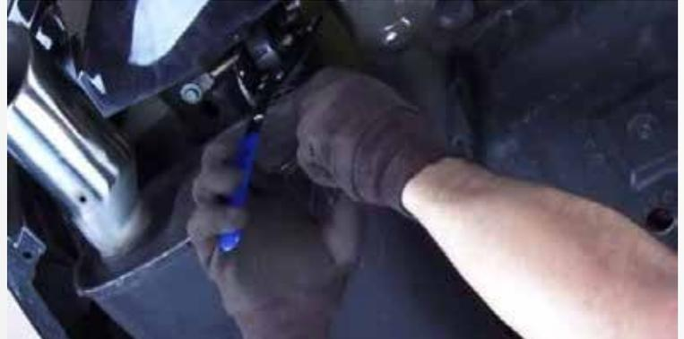
Using a pry bar or grommet removal tool, remove the rubber grommet located by the muffler tip from the muffler hanger.
