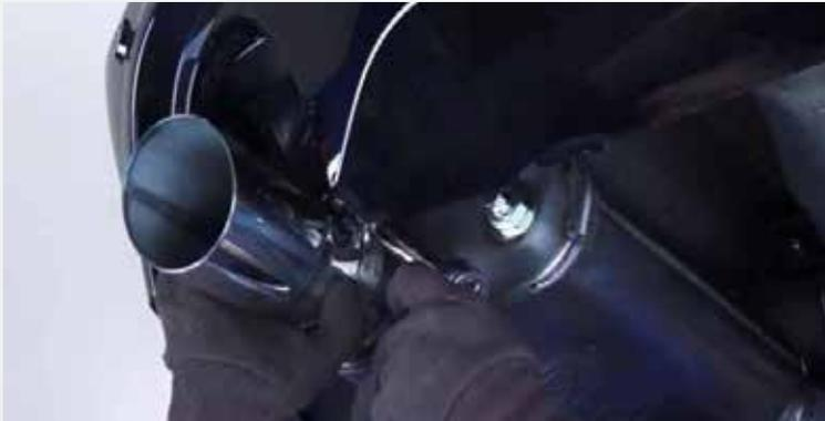
Slide and snug the exhaust tip onto the outlet tube of the muffler.
