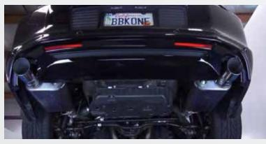
With all the clamps snug, make any fitment adjustments starting at the front clamps on the mid pipe and ending at the muffler tips, then tighten.
