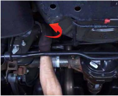
Twist the mid pipe so the muffler has enough clearance to be removed.
