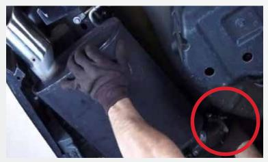
Slide the muffler towards the front of the vehicle and remove.
