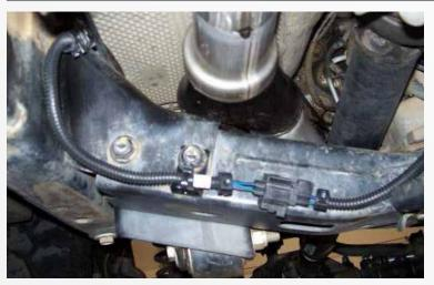
Using the oxygen sensor extensions reconnect all of the oxygen sensors. Zip tie the Y-Pipe oxygen sensor extension away from the exhaust along the cross member.
