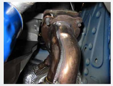
Remove the (4) 15mm nuts on the passenger side and driver side that secure the catted down pipe to the exhaust manifold.
