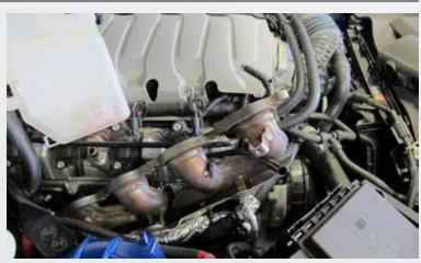
Remove the (5) bolts that secure the exhaust manifold to the cylinder head and remove it from the vehicle. NOTE the dip stick will come out with the exhaust manifold.
