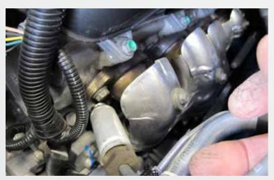
Remove the (4) spark plug wires from the coil packs and spark plugs.
