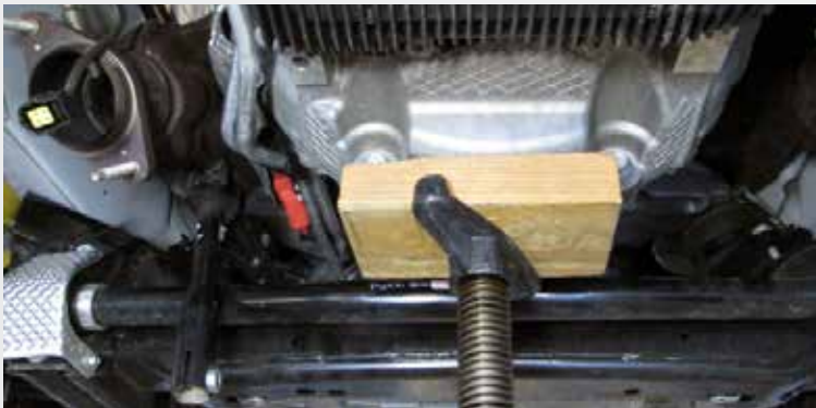
Safely support engine for removal and install motor mounts.
