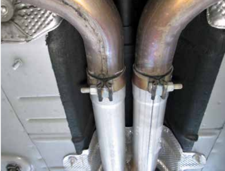
Using 15mm socket disconnect and remove factory head pipes.
