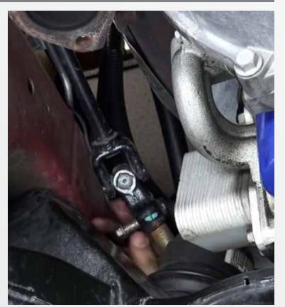
Remove the bolt on the steering u-joint at the rack and pinion shaft. Slide the shaft up into itself. Position the headers onto the head from underneath the vehicle and install 2 bolts to hold it in place.
