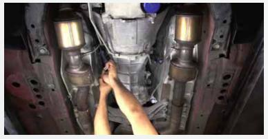
Loosen the clamps on the rear of the cat pipes and unplug the oxygen sensors at the transmission. Remove the flanged nuts at the collectors of the stock manifolds.
