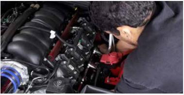
Position the cat pipes into the rear barrel clamps and up to the headers and install the provided 12 point head 10mm bolts. Tighten the collector bolts tight, then tighten the rear barrel clamps on the exhaust pipes
