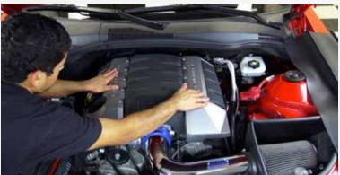
Reinstall all 4 oxygen sensors, the steering shaft, dipstick tube, spark plugs and wires, and the engine cover. Reconnect the negative battery terminal and start the engine to check for leaks. After about 100 miles of driving re-check the headers bolts and collector bolts.
