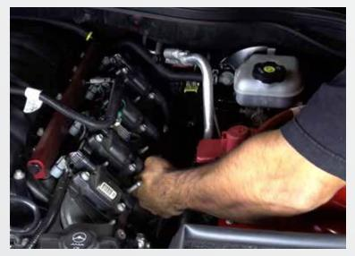
Remove the spark plug wires, spark plugs, and dipstick tube. Unplug the oxygen sensors at the back of the engine. Jack the car up and support on jack stands.
