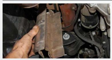
Remove the four nuts that hold the heat shields to the exhaust manifolds and remove them.
