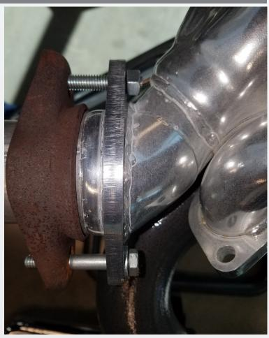
Now work the exhaust forward: torque the headers and installed supplied hardware. Notice in the picture on driver-side we supplied 1pc X 2 inch long bolt and 3pcs X 2 ½ Inch long bolts. Use the shorter 2 inch on the in-side of the elbow area. Now tighten exhaust down evenly and re-connect 02 sensor plugs.
