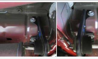
Remove the 2 bolts on the driver side and passenger side that hold the muffler mount to the chassis.
