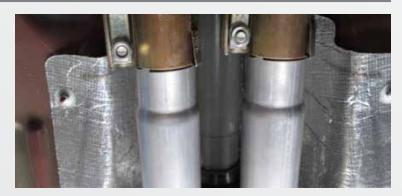
With the BBK Cat Back System install on the vehicle. Level out the BBK X-Pipe adapter and push it all the way forward towards the front of the vehicle and tighten down the stock 2 1/2" barrel clamps.
