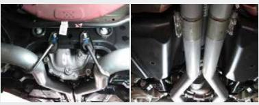
Install the 2 rear differential cross member mounts onto the BBK Under-Axle pipes. Using the (2) 3" couple supplied in the kit slide them onto the BBK X-Pipe adapter.
