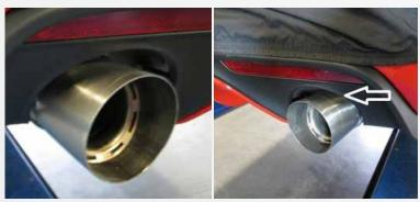
Slide the 3 "band clamp onto t the exhaust tip, then slide the exhaust tip onto the outlet tube of the muffler.
