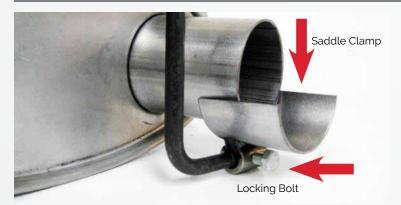
Use the hanger and saddle clamp for the outlet of the muffler. Slide the hanger through the corresponding rubber grommet on the chassis then snug the hanger into the saddle clamp and tighten the locking bolt to hold the hanger in place.
