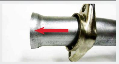
Slide the flared flanges over the head pipes so that the flared end of the flanges match the flared end of the head pipes as shown.
