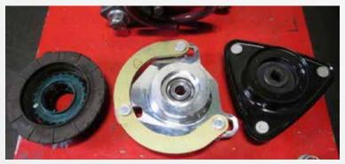
Place the Caster Plate on top of the bearing plate. Make sure that the raised lip around the bearing plate protrudes up through the center slot of the Caster Plate.
