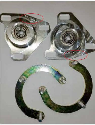
Determine which Camber/Caster Plate is driver or passenger side by looking at the engraved Sub2553-D for Driver side and Sub2553-P for Passenger side. Install the 2 provided stud plates from the bearing plate, with the studs protruding through the slots. NOTE! Make sure the larger radius between the 2 studs of each plate face the bearing.
