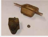
Remove nut from snubber stud and remove snubber from bracket.
