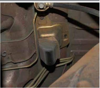
Locate pinion snubber bracket mounted to vehicle floor just above the front of the rear axle at the center of the vehicle.
