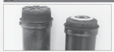
Remove stock dust boot and modify using a grinder or delete (See Photo). If strut was removed, re-attach to spindle now.
