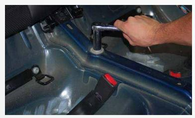
From under the car, remove the (2) #50 Torx bolts that retain the gas tank straps. Let fuel tank hang down onto drive-shaft.
