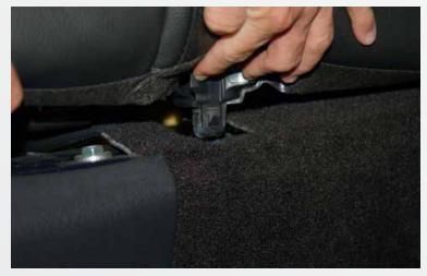
From inside the car, remove rear seat by pushing in on tabs under seat front, one on each side. Lift seat bottom up and remove from car.
