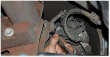
Remove clip for e-brake cable at caliper. Remove cable from actuating arm.
