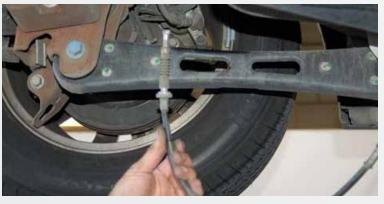
Slide cable out and through lower control arm. Let the cable hang.
